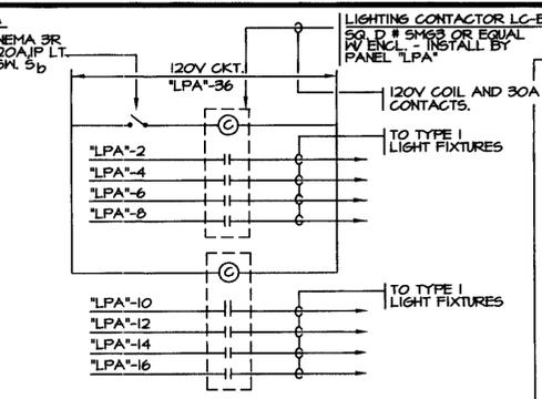
LC-B CONTROL WIRING DIAG.
