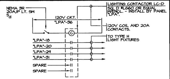
LC-D CONTROL WIRING DIAG.
